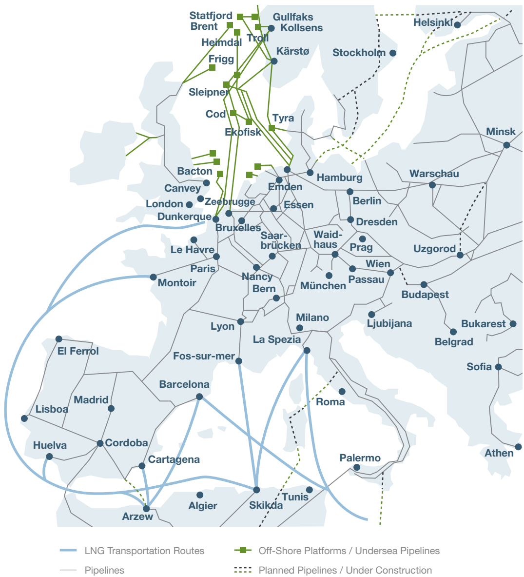
Figure 7: Most important gas pipelines and LNG transportation routes in Europe [Erdgas 2006]
