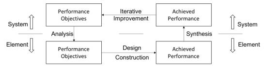
Figure 2: System- and element-level performance-based design process.
